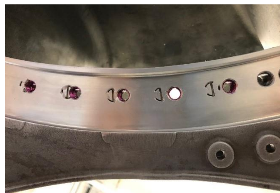
Result: Asymmetric bolt hole pattern
