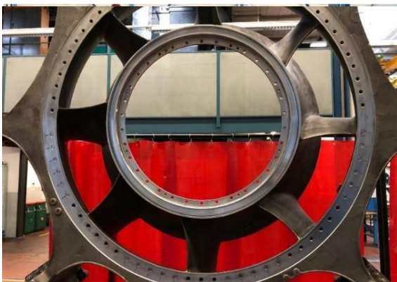
Plugging of old bolt hole pattern
