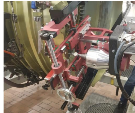
Repair 035 A1 Flange Bushing Repair - in-situ application of mobile mill.
