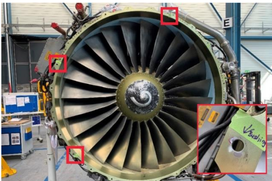
Repair 035 A1 Flange Bushing Repair - in-situ application of mobile mill.
