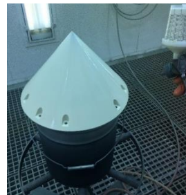
Step 4: Anti Erosion Paint
