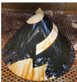
Step 1: Stripping of old paint
