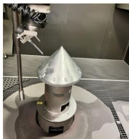
Step 2: Shot peening with robot
